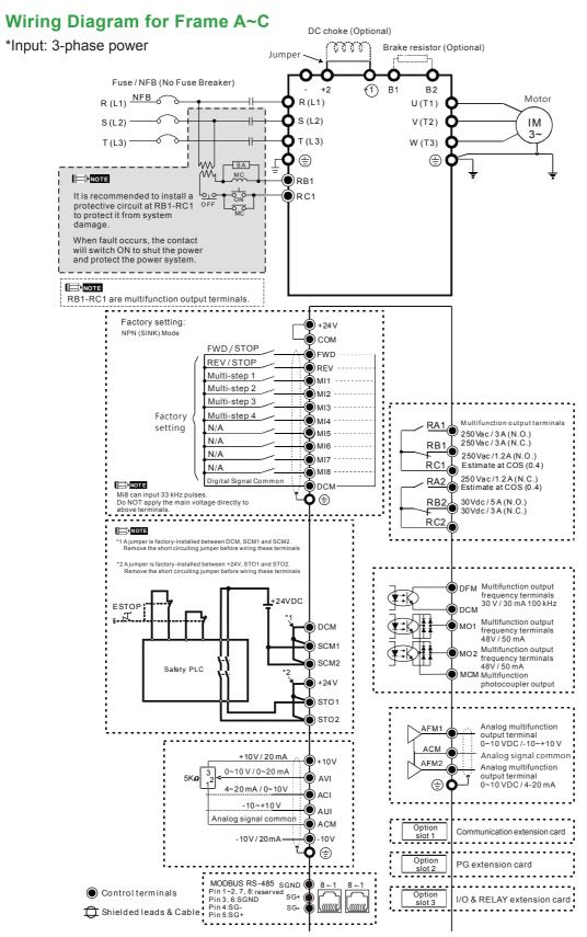
Note: It is not recommended to use a power capacitor or automatic power factor regulator (APFR) at the power input side. If the system requires such a device, please make sure a reactor is installed between the drive and the power capacitor or APFR.
